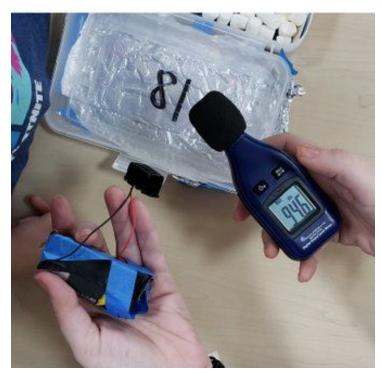
In another group, a student takes a baseline decibel measurement of the Piezo buzzer before packing it inside their pencil box to test their design which used stale marshmallows and aluminum foil.
