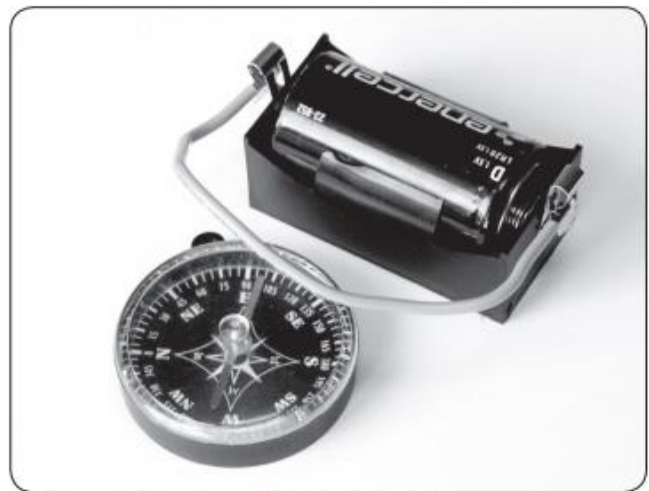
Electric current flows through the wire, turning it into an electromagnet. The magnetic field around the wire interacts with the needle in the compass, causing it to move.
