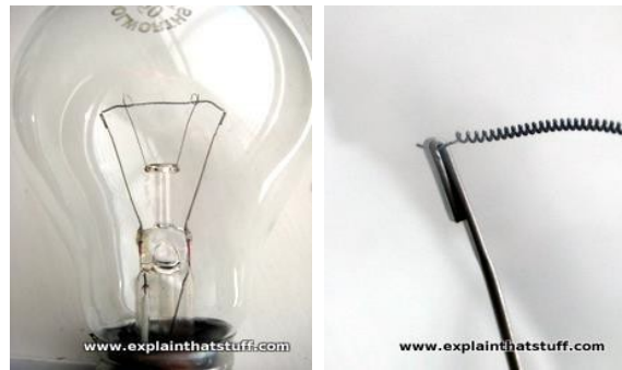
Photo: A modern, electric incandescent lamp. Left: The filament is a length of tightly coiled tungsten metal stretched between two terminals that let the current flow
